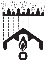
Stainless steel burners and radiant combination creates a searing hot grate temperature.
